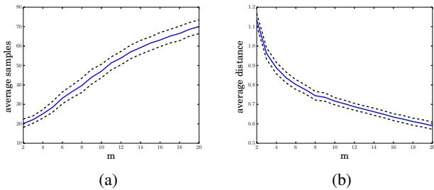
Fig. 4: Simulated average (a) samples required for convergence and (b) distance traveled for PQS algorithm with probability of error  $p = 0.1$ .
