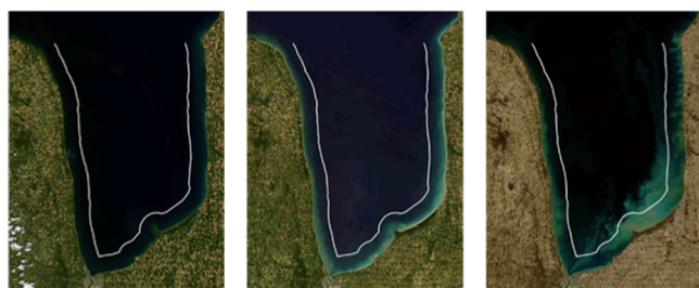
Figure 2. MODIS images of sediment resuspension in southern Lake Huron. Coded as none (left), moderate (center) when the sediment is inside the buffer line (white), and large (right) when extending offshore of the buffer line.
